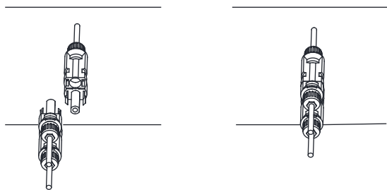
Pic 5.6 DC input connection
