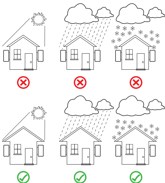
Pic 4.1 Recommended installation place
