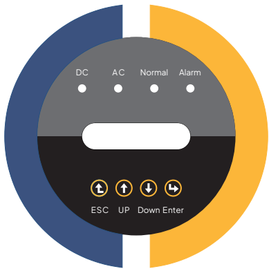
Pic 3.1 Front panel display
